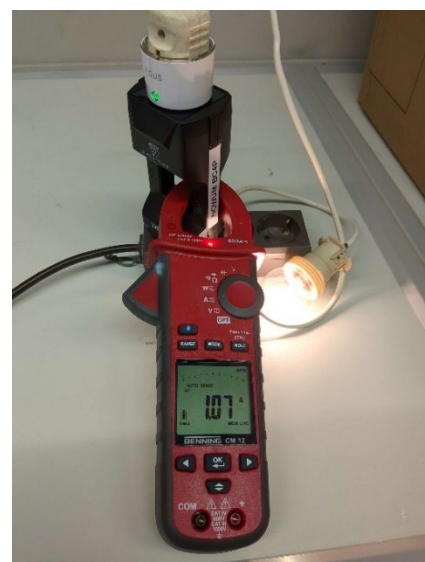
Figure 6. Image of the calibration process usage a power clamp and a known 60W light bulb
