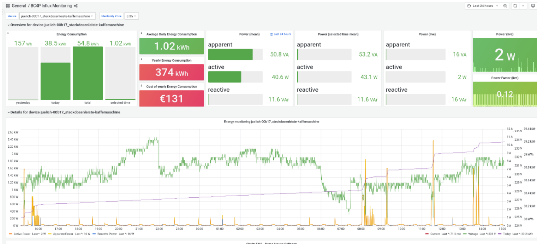
Figure 2 Dashboard providing stats of single measured devices as well as economic metrics (annual cost)
